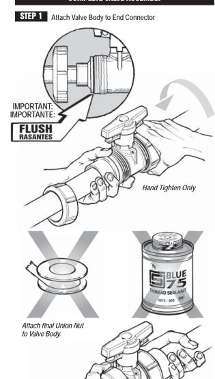
BE SURE THAT THE FACE OF THE END CONNECTOR SOCKET IS SQUARELY ALIGNED (FLUSH) WITH THE VALVE BODY AND IS FLUSH AGAINST THE O-RING. DO NOT USE THE REMAINING UNION NUT TO DRAW TOGETHER ANY GAPS BETWEEN THE END CONNECTOR AND THE VALVE BODY.
