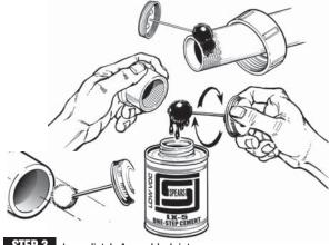
STEP 3 Immediately Assemble Joint
