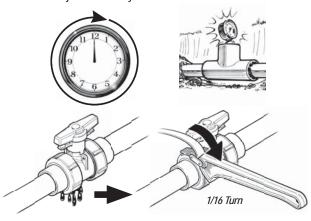
DO NOT OVER TIGHTEN AS DAMAGE MAY OCCUR
