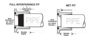
Do not use components which do not properly mate.
